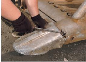
A standard prying tool is used to disengage the "latch" for removal of the **hammerless** retainer.
